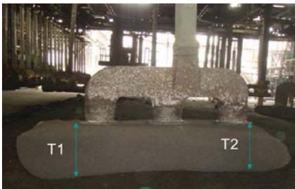
Figure 3. Anode butt thickness measurement
