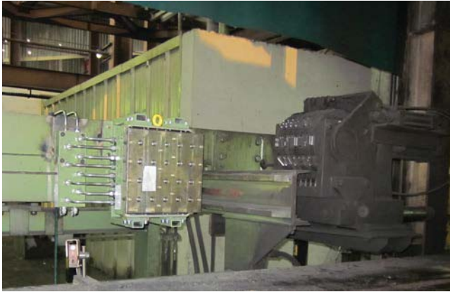
Figure 5: Dot Code Stamping unit at AM
