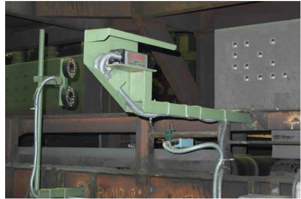
Figure 6: Camera & IR light source at rodding station, capturing the baked anode
