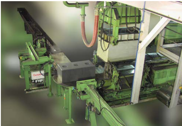
Figure 7: Anode push-off at vibrocompactor
