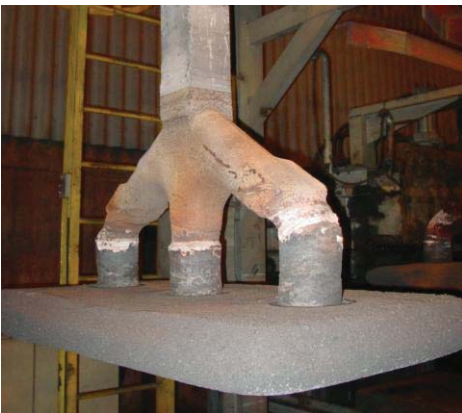
Figure 4. Excellent example of a well cleaned carbon anode butt.
