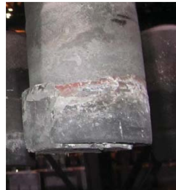
Figure 5. Cast iron adhered to stub after thimble stripping process.
