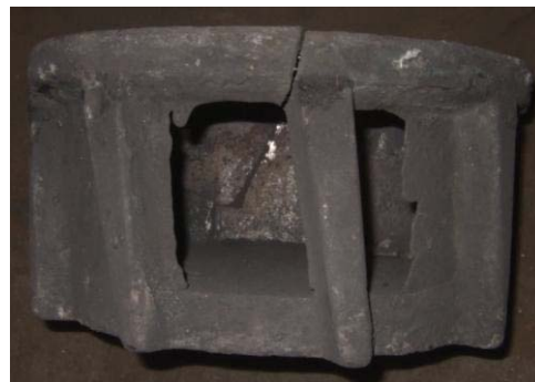
Figure 7. A 'cold shut' in a cast iron thimble.
