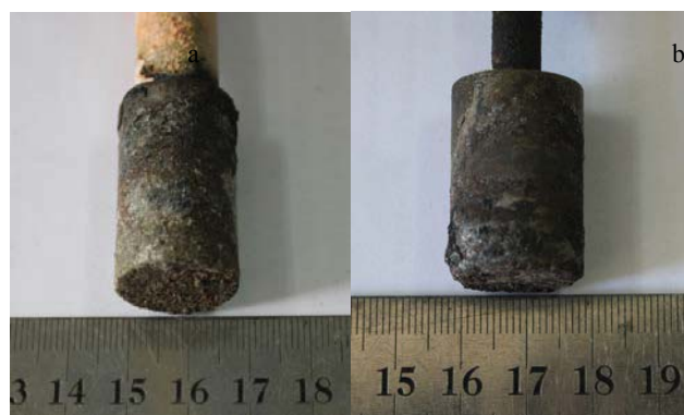
Figure 4. Photographs of the alloy anodes after aluminum electrolysis at 950 °C
