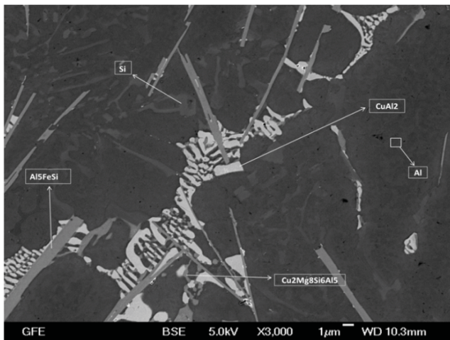
Fig. (5) BSE image of 1% Al 2 O 3 cast in semi-solid state showing the main microstructure constituents appearing in the as-cast state.
