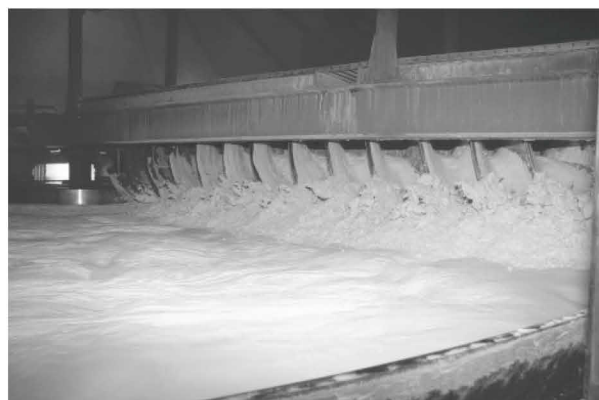
Figure 1. AOS pan filter, discharge scroll
