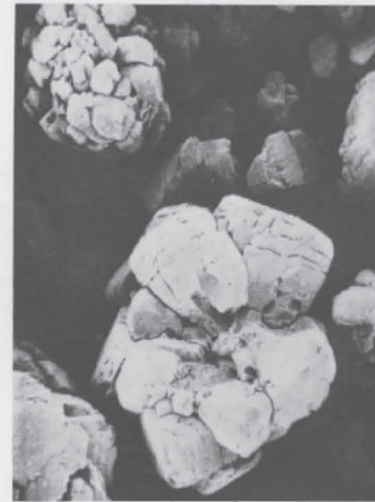
(b). Aggregate: Shape factor = 0.744 Blockiness index = 0.480
