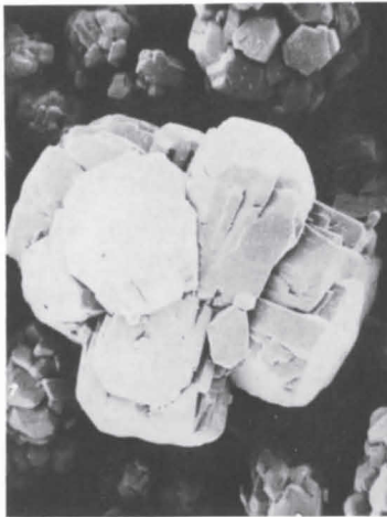
(b). Aggregate: Shape factor = 0.769 Blockiness index = 0.695
