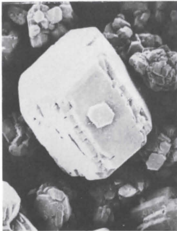
(a). Blocky crystal: Shape factor = 0.841 Blockiness index = 8.12
