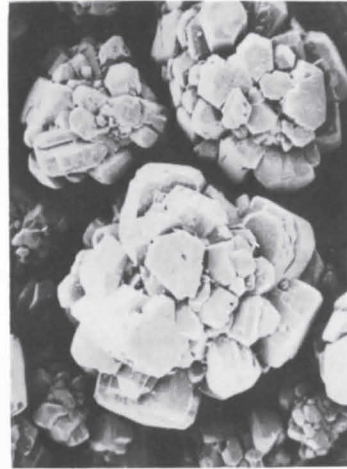
(c). Agglomerate: Shape factor = 0.758 Blockiness index = 0.246
