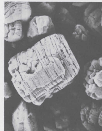
(a). Blocky crystal: Shape factor = 0.843 Blockiness index = 11.2
