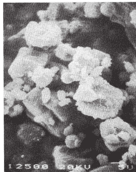
Figure 10. S.E.M. micrographs of typical alumina dusts collected with the Perra pulverimeter (2000 X).
