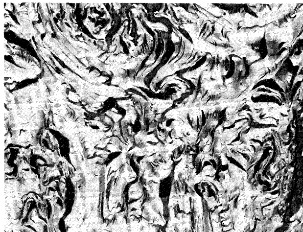
Figure 2. Coke from decant oil. Bent and curved laminae. (Mag. 100X)
