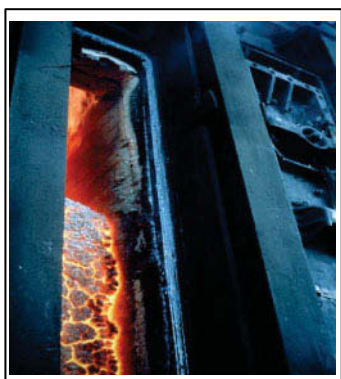
Figure 3. Coke Oven Tunnel Head
