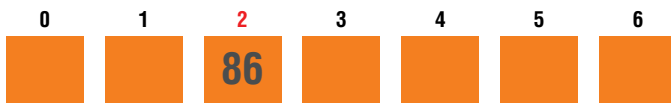
Figure 13.2: To store 86 in the hash table, you perform modulo by the number of slots and get 2.
