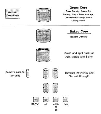
AP=Air Permeability, AR=Air Reactivity, CO2=CO2 Reactivity, CS=Compressive Strength TC=Thermal Conductivity, TS=Thermal Shock, YM=Youngs Modulus
