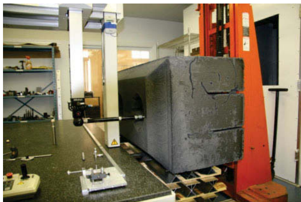
Figure 1 : Set-Up of the stub holes measurements with the CMM
