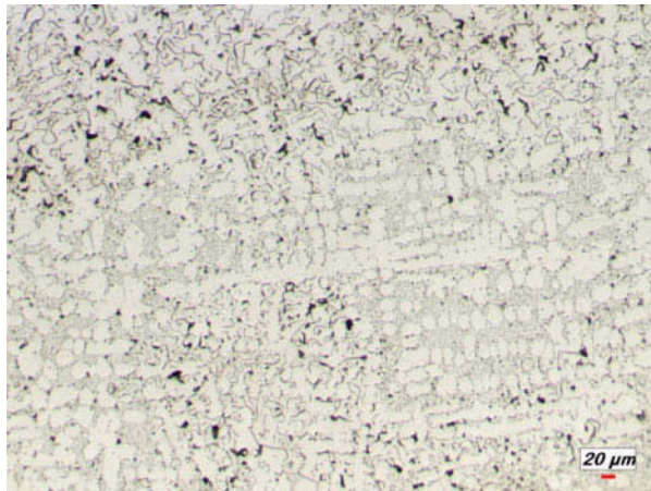
Figure 11 : Microstructure of the cast iron at TC I1 location
