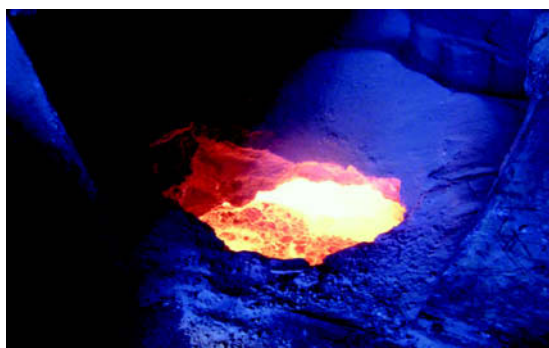
Figure 1: The level of dusting evaluated in the tapping hole, in this case a dusting index of 2.
