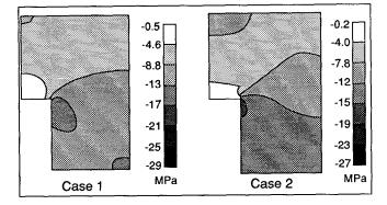
Figure 6. Compressive stresses in the bottom block without (Case 1) and with a 2.5 cm (Case 2) layer of graphite powder between the bar and the slot bottom.
