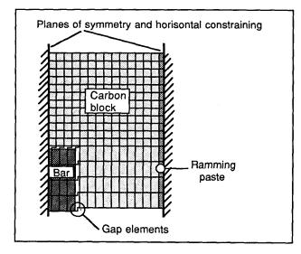
Figure 2. The 2-dimensional model for stress analysis.
