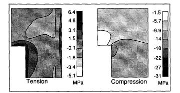
Figure 10. Stress fields caused by high friction between collector bar and carbon block (Case 6).
