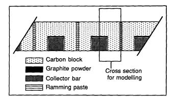
Figure 1. Cross section of part of the carbon bottom pane shows the selected part for modelling,
