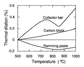
Figure 3. Thermal dilation of current collector bar, carbon block and ramming paste in the temperature range between paste baking (≈500°C) and cell operating temperature.
