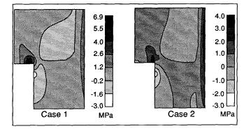
Figure 5. Tensile stresses in the bottom block without (Case 1) and with a 2.5 cm (Case 2) layer of graphite powder between the bar and the slot bottom.
