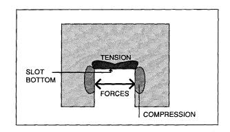
Figure 4. Stress zones caused by the forces acting between the collector bar and the carbon block.
