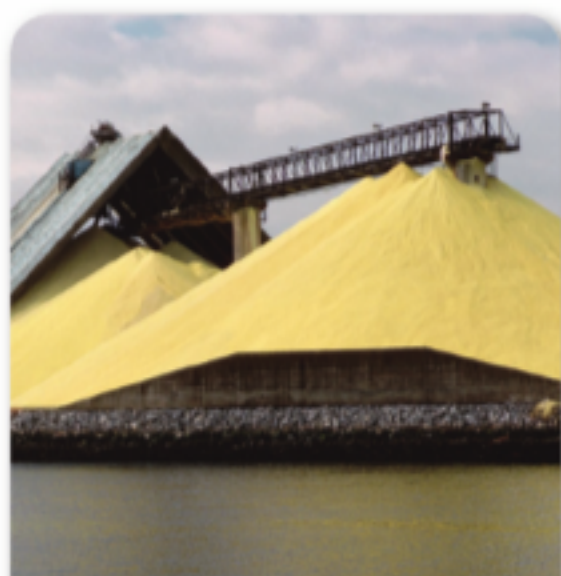
Figure 9 Sulfur, such as these piles at Vancouver Harbor, can be extracted from petroleum products by a chemical process. Sulfur is also mined by forcing hot water into underground deposits and pumping the liquid sulfur to the surface.
