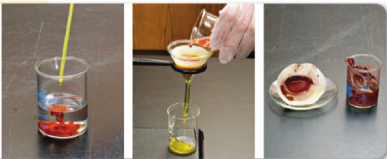
Figure 8 Silver chromate is formed when potassium chromate is added to silver nitrate. Note that not all of the precipitate can be removed from the filter paper. Still more of the precipitate is lost because it adheres to the sides of the beaker.
