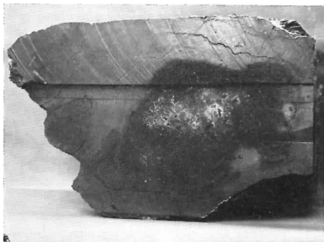
Fig. 6. Cut section of used cathode block showing coring.
