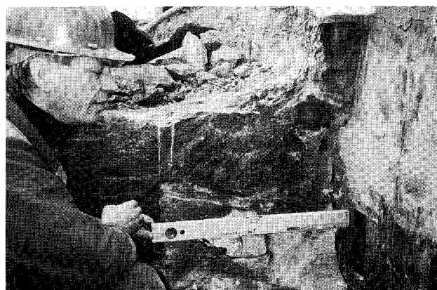
Figure 14. Forced tilt of carbon side lining filler block following bottom heave in cathode with strongly supported steel shell. The vertical displacement is 7.5 cm measured from bottom corners of filler block. Pot life was 1032 days.
