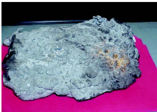
Figure 7: Surface of the metal leftover peeled off the graphitized cathode of the stopped pot: the molding shows the holes on the cathode's surface.
