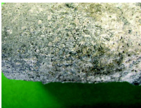
Figure 4: Course, grainy topography of electrolyzed graphitic cathode material
