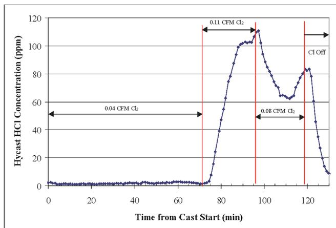
Figure 8. HCl emissions from Hycast (Test 4a)
