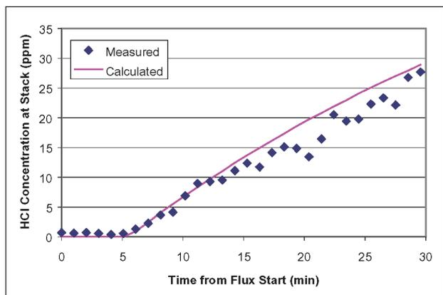
Figure 7. Calculated chloride emissions for Test 3a
