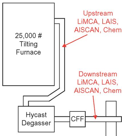
Figure 1. Casting Station
