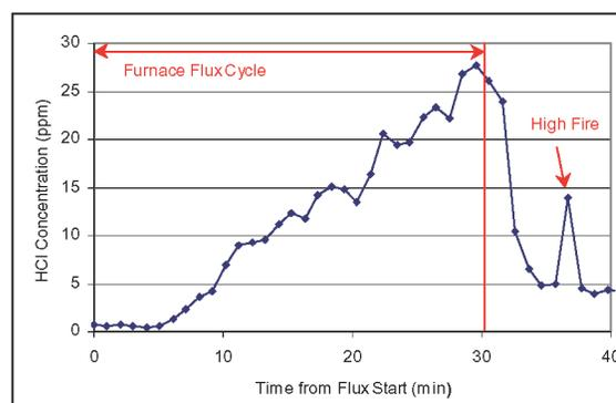
Figure 4. HCl Concentration in the Furnace Stack During Ar-Cl Furnace Flux (Test 3a)
