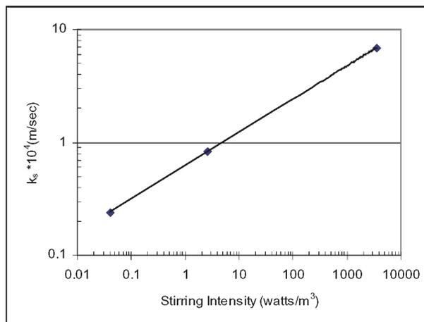
Figure 6. Rate constant for surface oxidation,  $k_s$ , as a function of stirring intensity
