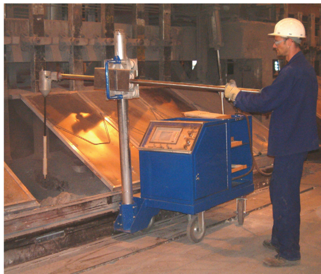
Figure 12: “Manipulator” equipment for easy liquidus measurements
