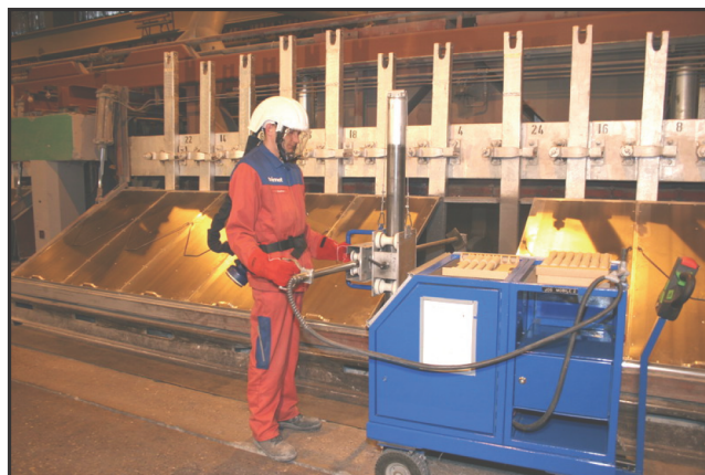
Figure 1: Superheat Measurement in Reduction Cells
