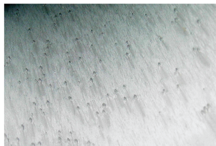
Figure 6: Typical fouling layer with a thickness in the range of 1 mm.
