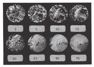
Fig.6 - Successive sections of a sample containing l w/o Fe. Figures indicate distance in mm from the lance tip. Sample diameter 20 mm.
