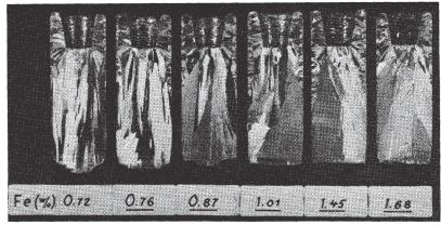
Fig.3 - Sample series from the Al-Fe system. Length of samples 60 mm.
