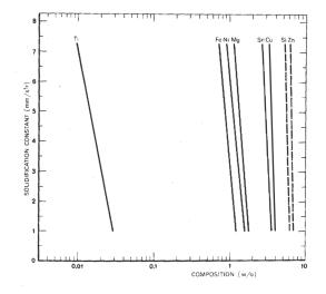
Fig.5 - Critical composition of all feathery crystalproducing elements at different solidification constants. All basic data from Table 1.
