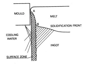
Fig.7 - Schematic illustration of the possible sites (A and B) where twins can be nucleated in DCingots.
