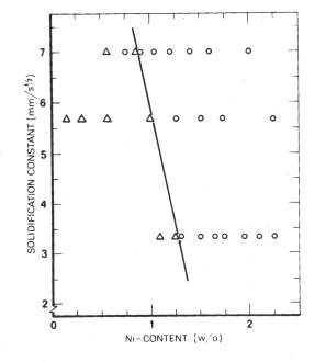
Fig.4 - Sample structures in the Al-Ni system as a function of composition at different solidification constants. Triangles = no feathery crystals, circles = feathery crystals.
