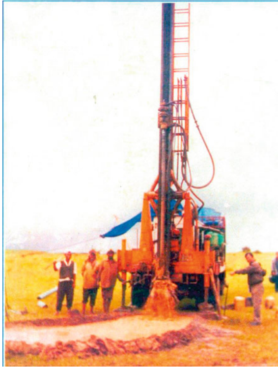
Fig. 2.1 DTH rig in action
