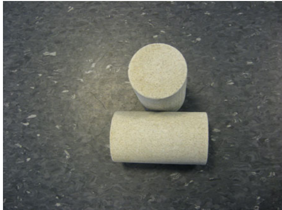
Fig. 3.12 Two Berea Sandstone core-plugs taken from quarried blocks
