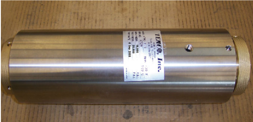
Fig. 3.6 The Temco biaxial core-holder used during the core-flooding experiments
