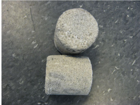
Fig. 3.11 Two sandstone core-plugs drilled in horizontal direction from whole-cores taken from Waarre C formation in the Naylor Field
