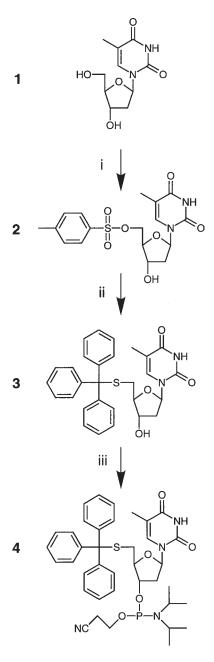
Fig. 2. Synthesis scheme for 5'-S-trityl, 3'-*O*-(2-cyanoethyl-*N*,*N*-diisopropylamino) thymidine. i. *p*-Toluene sulfonyl chloride. ii. Sodium salt of trityl mercaptan. iii. Diisopropylelthyl amine, 2-cyanoethyl *N*,*N*-diisopropylchlorophosphoramidite. *See text* for details.
