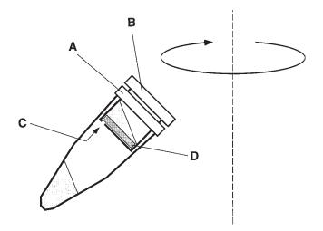
Fig. 1. Setting for spin filtration through glass fiber filters. (A) Regular 1.5-ml microcentrifuge tube. (B) Push-in cap with a concavity deep enough to hold at least 100  $\mu$ L. (C) Small hole pierced with a needle at the bottom edge of the cap concavity. (D) Whatman GF/C glass fiber filter 6 mm in diameter.
