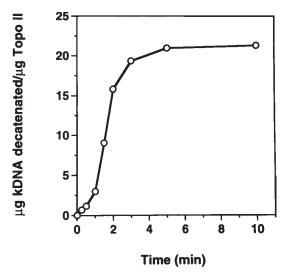
Fig. 1. Decatenation of  $[{}^{3}H]kDNA$  by purified topoisomerase II $\alpha$  isolated from human small-cell lung cancer H209 cells. In this experiment, the decatenation of 0.7 µg  $[{}^{3}H]kDNA$  (20,000 cpm) by 31 ng purified topoisomerase II $\alpha$  at 1 m*M* ATP and 100 m*M* NaCl was assayed over a time range of 15 s to 10 min. The linear part of this curve shows that the rate of decatenation for this enzyme preparation is about 6 µg kDNA decatenated/µg topoisomerase II/min.
