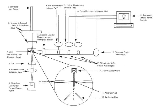
Fig. 1. Schematic diagram of a typical flow cytometer.
