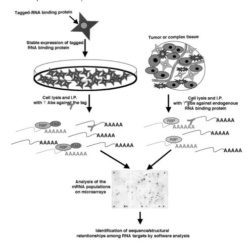
Fig. 1. Schematic of ribonomic analysis. Tagged or endogenous mRNA-protein complexes (mRNPs) are isolated from cell lines or a complex tissue such as a tumor. The mRNAs associated with the targeted mRNP complexes are then characterized by using an en masse assay, such as a cDNA microarray. Sequence and functional relationships amongst the detected mRNA targets and the protein products they encode can then be investigated.
