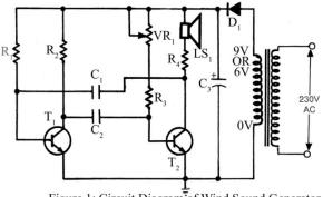
Figure 1: Circuit Diagram of Wind Sound Generator
