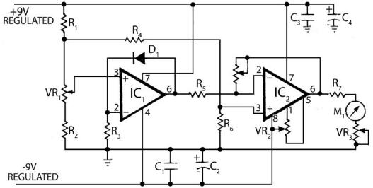
Figure 1: Circuit Diagram of Electronics Thermometer
