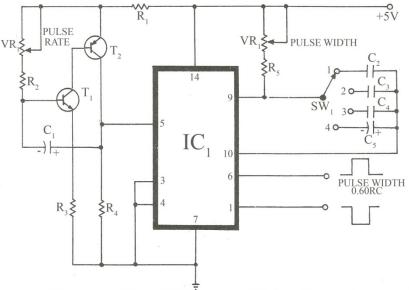
Figure 1: Circuit Diagram of Pulse Generator
