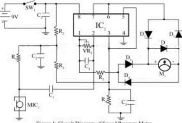
Figure 1: Circuit Diagram of Sound Pressure Meter
