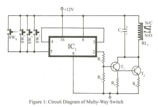
There is no need to connect a debouncing circuit between the switches and the IC. PARTS LIST Resistors (all ¼-watt,  $\pm$  5% Carbon) R1 = 10 KΩ; R2 = 3.3 KΩ; R3 = 1 KΩ; R4 = 10 Ω Capacitor C1 = 50 µF/25V Semiconductors IC1 = CD4042A; T1 = BC107; T2 = SL100 Miscellaneous SW 1 – SWn = Push to on switch; RL1 = 12V, >100 Ω relay
