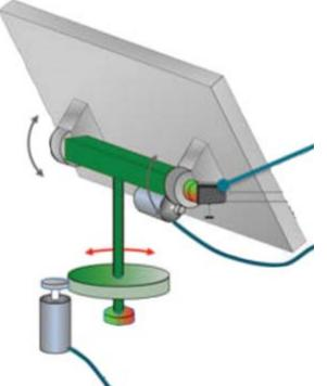
Similarly, LDR3 and LDR4 track the sun along Y axis. Fig. 2 shows the proposed assembly for the solar tracking system.
