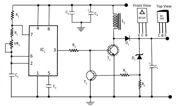
PARTS LIST Resistors (all <sup>1</sup>/<sub>4</sub>-watt,  $\pm$  5% Carbon) R1, R2, R5 = 10 KΩ; R3, R4 = 220 Ω 1/2-watt; VR1 = 47 KΩ Capacitors C1 = 0.0047 µF; C¬2 = 0.01 µF; C3 = 0.1 µF; C4 = 470 µF/25V; C5 = 2200 µF/35V Semiconductors D1 = 1N4007; D2 = Zener 12V, 500mA <sup>1</sup>/<sub>2</sub>-watt; T1 = BC549; T2 = BD139; IC1 = NE555 timer IC Miscellaneous L1 = 100 Turns, 24 SWG insulated copper wire on 40mm Dia. toroidal core
