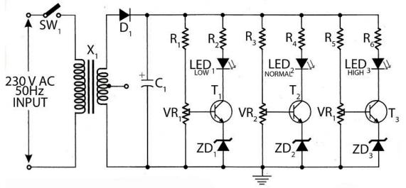
Figure 1: Circuit Diagram of Mains Voltage Indicator
