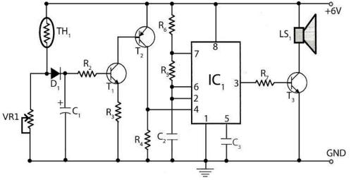
Figure 1: Circuit Diagram Of Fire Alarm Using Thermistor
