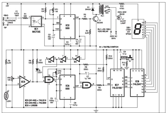
The telephone lines (TIP and RING) Counter 74LS192 (IC7) is reset to zero state by making its reset pin 14 high through reset switch S1. The 7-segment, common-anode display DIS1 is driven through IC 74LS47 (IC8). When the phone rings, count '1' is displayed after nearly one minute. This happens if the watchman fails to focus the torchlight beam on LDR1.
