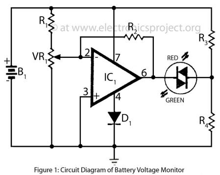
All rechargeable battery has their specific level of charging and discharging, they are likely to get damage if the battery voltage exceeds that level. Here is a simple circuit battery voltage monitor used to indicate the state of battery by monitor them.
