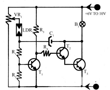
Figure 1 : Circuit Diagram of Flashing Light With Twilight Switch
