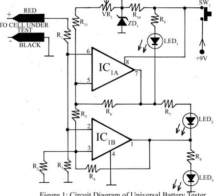
Figure 1: Circuit Diagram of Universal Battery Tester
