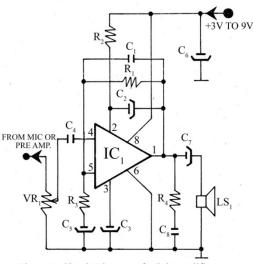
Figure 1: Circuit Diagram of Mini Amplifier
