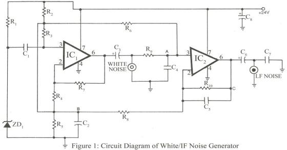
PARTS LIST Resistors (all  $\frac{1}{4}$ -watt,  $\pm$  5% Carbon unless stated otherwise) R1 = 470 KΩ; R2, R5, R8, R9 = 10 KΩ; R3, R6, R10 = 100 KΩ; R4 = 4.7 KΩ; R7 = 1 MΩ **Capacitors** C1 = 0.47  $\mu$ F; C2 = 100  $\mu$ F/10v; C3, C6 = 1  $\mu$ F/16v; C4 = 0.15  $\mu$ F; C5 = 0.015  $\mu$ F;  $C7 = 0.001 \ \mu\text{F}; C8 = 100 \ \mu\text{F}/25\text{V}$ **Semiconductors** IC1, IC2 = 741, ZD1 = 12V 400mW
