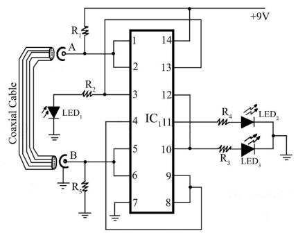
Figure 1: Circuit Diagram of Coaxial Cable Tester
