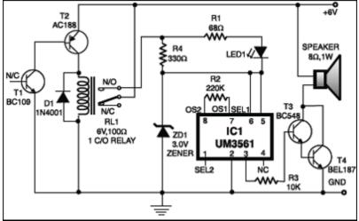
The second part of the circuit comprises popular IC UM3561 (a siren and machine-gun sound generator IC), which can produce the sound of a fire-brigade siren. Pin numbers 5 and 6 of the IC are connected to the +3V supply when the relay is in energised state, whereas pin 2 is grounded.
