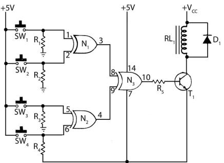
Figure 1: Circuit diagram of multi switch controlled relay
