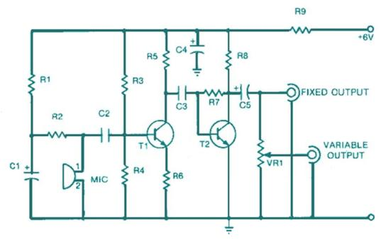
PART LIST RESISTORS R1=1.2 K $\Omega$ ; R2=2.7 K $\Omega$ ; R3=33 K $\Omega$ ; R4=6.8 K $\Omega$ ; R5=3.3 K $\Omega$ ; R6=100; R7=560 K $\Omega$ ; R8=4.7 K $\Omega$ ; R9=10 K $\Omega$ ; VR=11 K $\Omega$ TRANSISTORS T1=BC149C; T2= BC147B Capacitors C1=47 $\mu$ , 10V; C2,C3=0.1 $\mu$ ; C4=220 $\mu$ , 10V; C5=10 $\mu$ Miscellaneous BATT 6VOLT Battery MIC Condenser Microphone OTHERs PCB ,Connecting wires, hardware etc...
