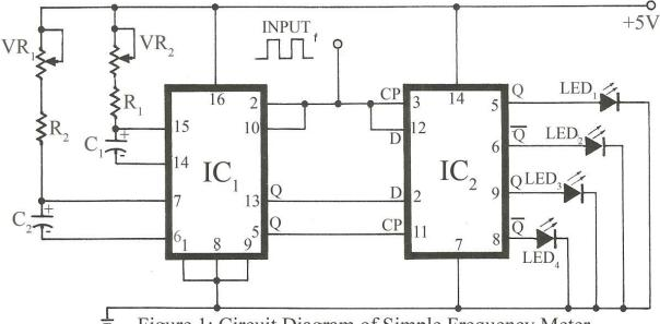
Figure 1: Circuit Diagram of Simple Frequency Meter
