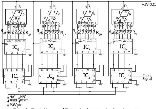
Figure 2: Circuit Diagram of Electronics Counter using Decade counter
