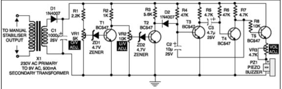
Some manual stabilisers available in the market incorporate the high-voltage auto-cut-off facility to turn off the load when the output voltage of manual stabiliser exceeds a certain preset high voltage limit. The output voltage may become high due to the rise in AC mains voltage or due to improper selection by the rotary switch on manual stabiliser.
