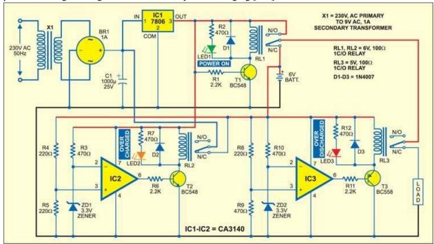
automatically shifts to DC when mains power fails. When mains power resumes, the load is again powered through the regulator and the battery starts charging [188].
