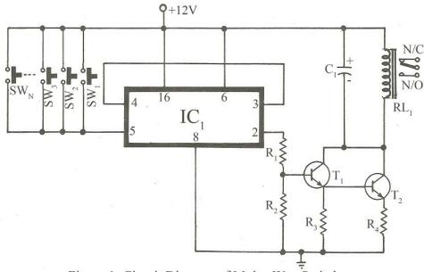
Figure 1: Circuit Diagram of Multy-Way Switch
