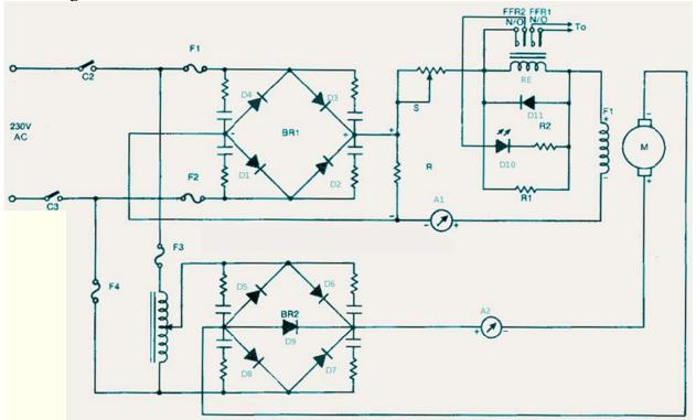
In case the motor field current fails due to any fault, the voltage drop across resistor (R1) will be zero which denergizes the relay (FFR) and cuts off the armature supply.
