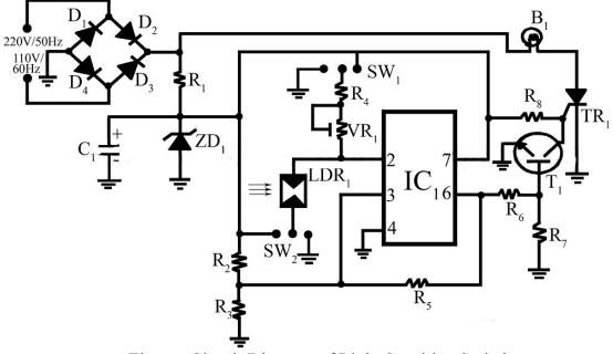
Figure: Circuit Diagram of Light Sensitive Switch
