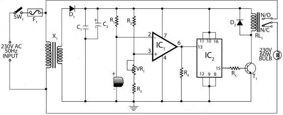
Figure 1: Circuit diagram of sound operated light
