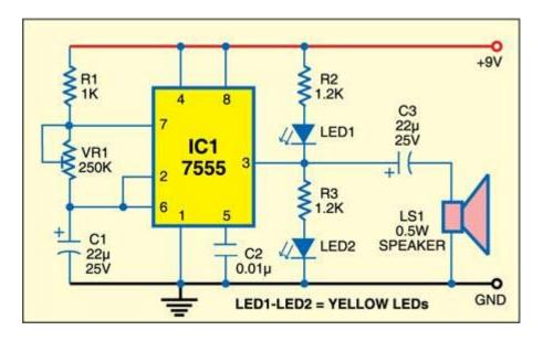
248. Clock Tick-Tock Sound Generator & LED Pendulum [246]
