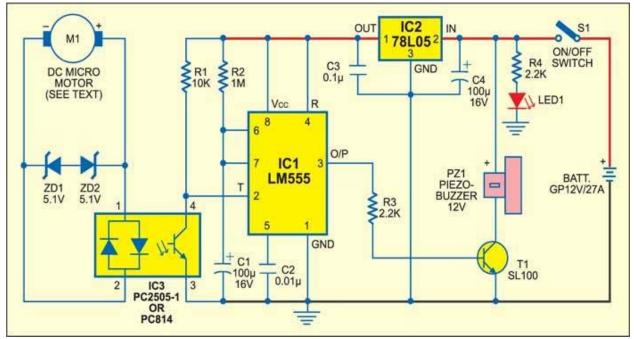
Power supply switch S1 should be kept 'on' when you are using this bicycle guard. When it is flipped towards 'on' position, the circuit gets power from the miniature 12V battery. Now LED1 lights up and resistor R4 limits the LED current. Next, the monostable built around IC1, which is CMOS version of timer LM555, is powered through a low-current, fixed-voltage regulator IC2 (78L05).
