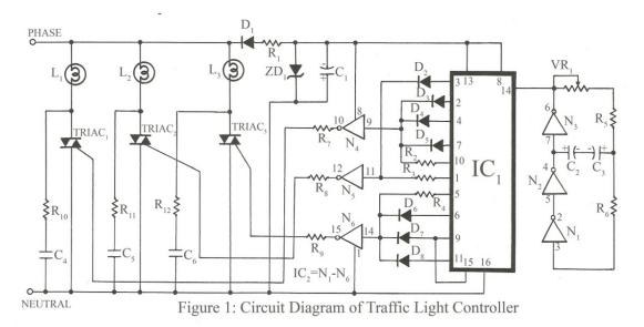
PARTS LIST Resistors (all ¼-watt, ± 5% Carbon unless stated otherwise) R1 = 5 KΩ/5W; R2, R3, R4 = 22 KΩ; R5 = 100 KΩ; R6 = 1 MΩ; R7, R8, R9 = 1 KΩ; R10, R11, R12 = 100 Ω/1W; VR1 = 1 MΩ Capacitors C1 = 1000  $\mu$ F/16V; C2, C3 = 22  $\mu$ F/16V; C4, C5, C6 = 00.1  $\mu$ F/400V Semiconductors IC1 = CD4017; IC2(N1 – N6) = CD4049; D1 = BY127
