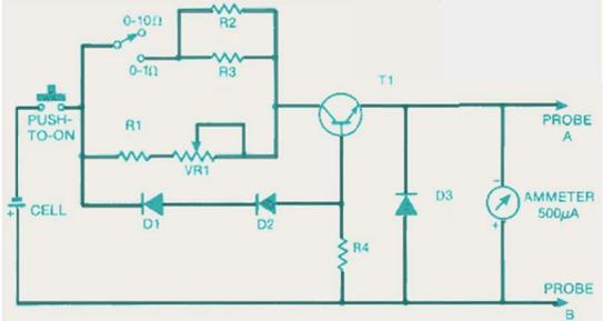
Part List RESISTORS R1=27K; R2=3.3K; R3=3.3K; R4=330K; VR1=100 OHM DIODES D1=1N4001; D2=1N4001
