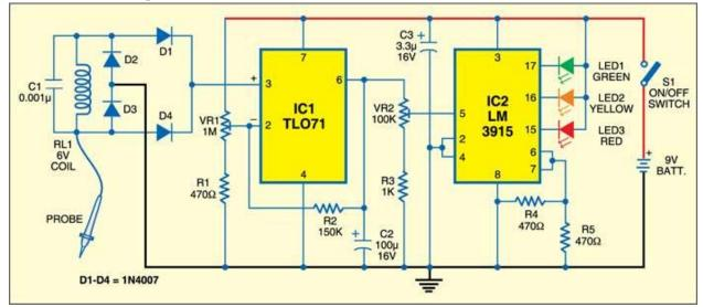
to the earth. An ordinary AC tester cannot detect the earth leakage if current is not high enough to switch on a neon lamp [118].
