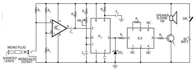
Figure 1: Circuit diagram of anti bag thief alarm
