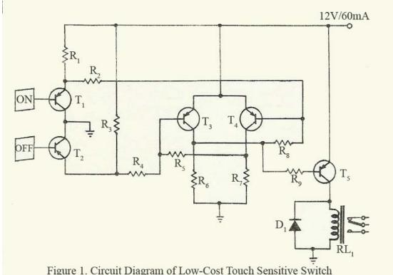
Figure 1. Circuit Diagram of Low-Cost Touch Sensitive Sw
