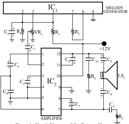
Figure 1: Circuit Diagram of Car Reverse Horn
