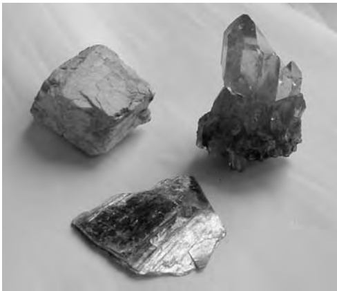
Figure 7.2 The components of granite: feldspar (top left), quartz (top right) and mica (middle bottom).
