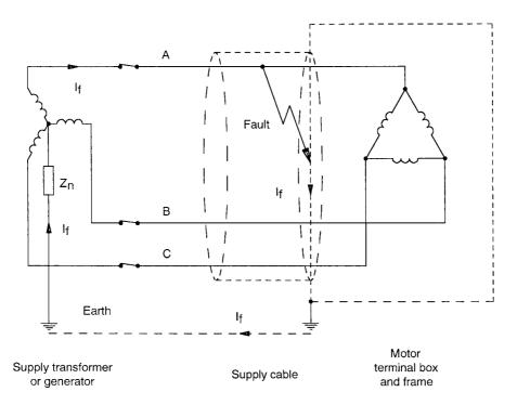
Figure 13.10 Earth loop impedance of a three-phase circuit.
