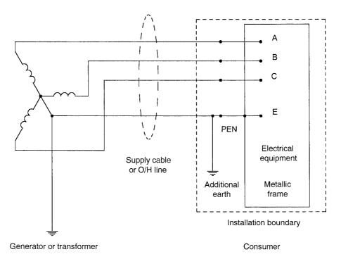
Figure 13.5 IEC earthing system type TNC.
