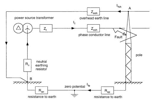
Figure 13.12 Earthing circuit of an overhead transmission route.
