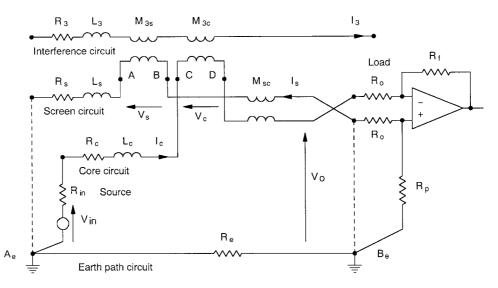
Figure 13.15 Interference and screening circuit of cables that are run in parallel with each other. The signal cable is terminated by an amplifier at the far end.
