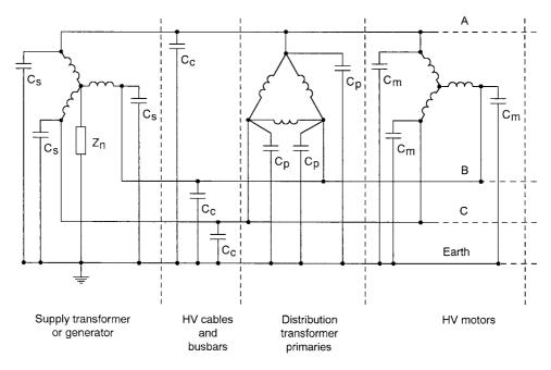
Figure 13.2 Earthing circuit of leakage capacitance in a high voltage system.
