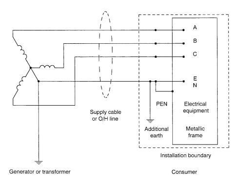
Figure 13.7 IEC earthing system type TNCS.
