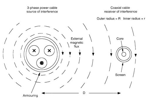
Figure 13.13 Mutual coupling between spaced out cables.
