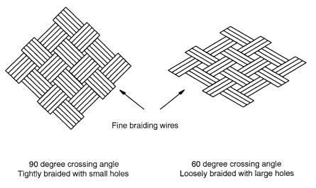
Figure 13.16 Holes in the braided armouring of instrumentation cables.
