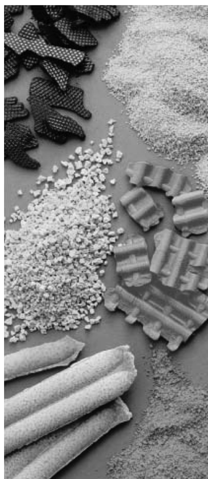
FIGURE 38.7 Examples of roller compactor output. (Courtesy: The Fitzpatrick Company.)
