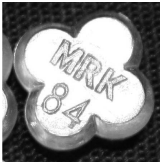
FIGURE 42.12 Example of a directly shaped tablet following a melt extrusion process illustrating the ability to form complex shapes, such as the Merck corporate logo (image weight ca. 200 mg).
