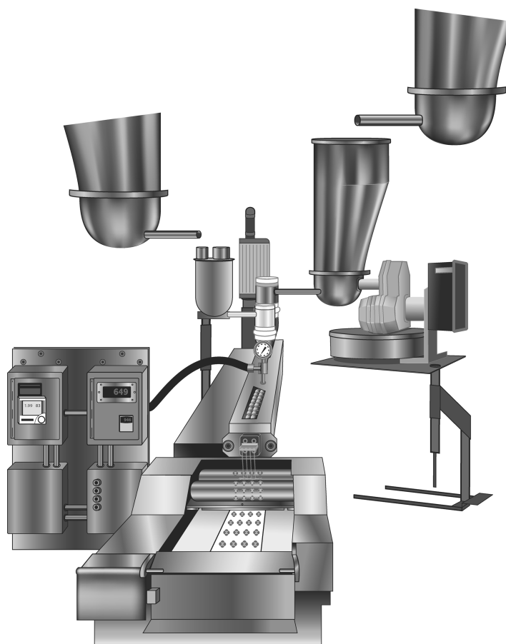
FIGURE 42.4 Direct-to-drug-product extrusion process train schematic, highlighting bulk feeders, precision loss in weight feeders, liquid injection, and calendaring of tablet between two chilled rolls.
