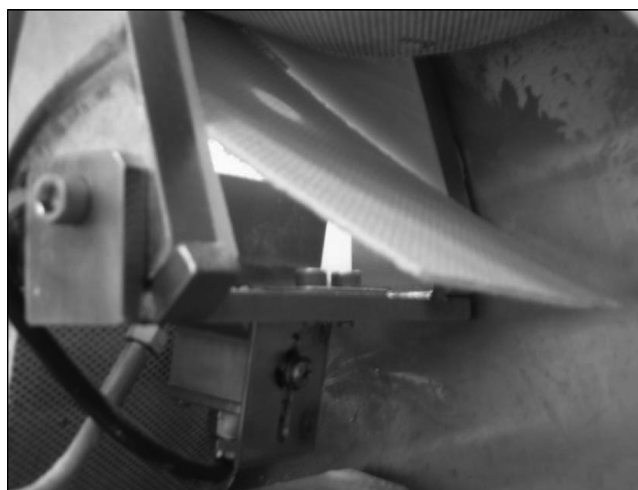
FIGURE 43.13 NIR measurement head installed in Gerteis Macropactor.
