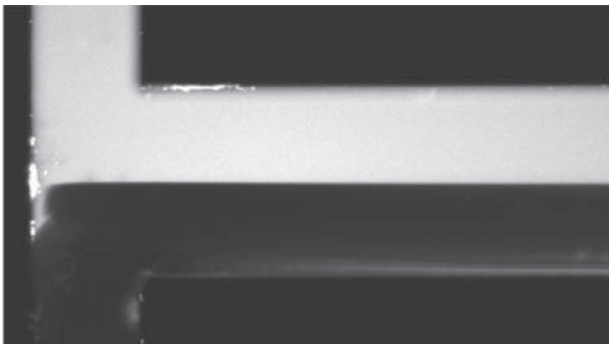
Figure 4.9 Parallel flow in a T-mixer ( 200 \times 100 \times 100 μm) system water/water rhodamin, T = 20 °C, Re = 120 [14]. (Adapted with permission from Wiley.)
