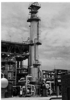
Figure 5.2. Example of a reactor using a heterogeneous catalyst in a fixed bed for the hydrogenation of fuels © IFPEN
