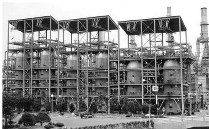
Figure 5.8. Industrial unit for hydrotreating petroleum in a fixed catalyst bed © M. Roussel, ScOpimag
