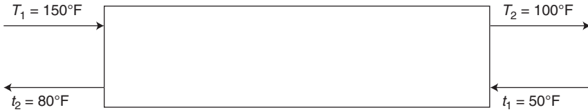
Figure 16.13 Ideal countercurrent heat exchanger; Illustrative Example 16.5.
