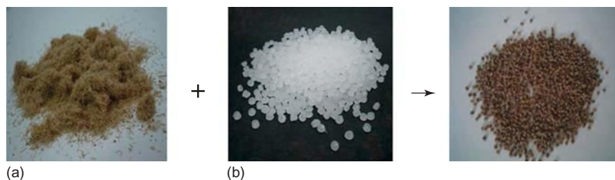
Figure 26.1 Typical composite components: (a) fiber, (b) polymer and additives. (See insert for the color representation of the figure.)
