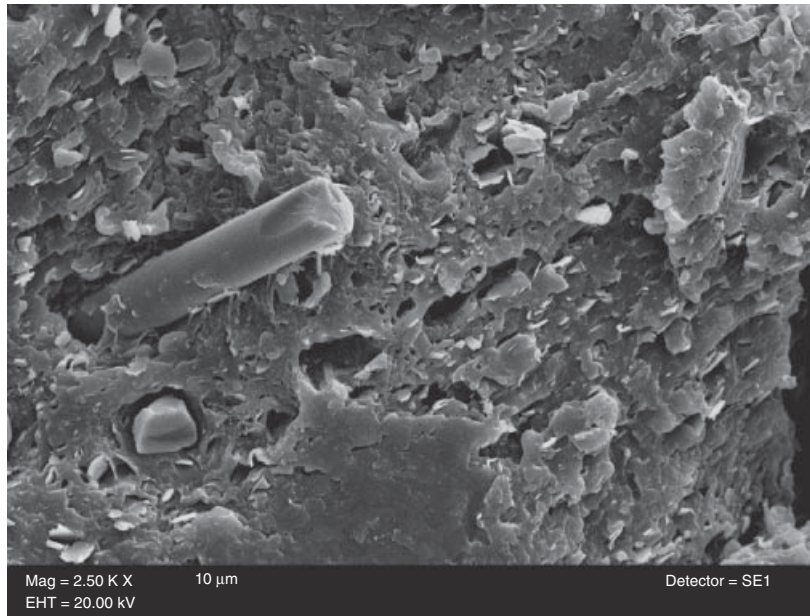
Figure 31.9 Mix of PP-PP-g-MAH with glass fibers. Adhesion between the fibers and matrix is poor.
