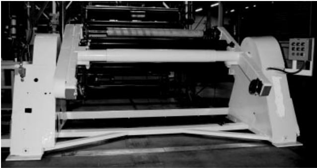
Figure 9.2 A turret winder used in the plastics industry.
