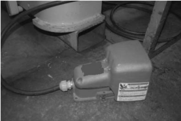
Figure 9.12 A shielded foot pedal control with a toe-kick will reduce the likelihood of inadvertent activation of a machine.
