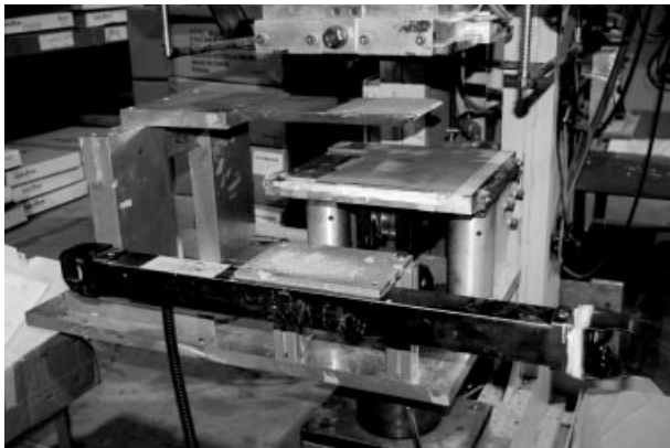
Figure 9.8 A two-hand control prevents activation of the machine until the operator's hands are clear of the danger area.
