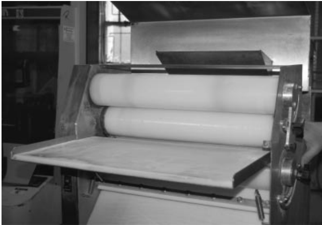
Figure 9.4 An interlocked guard over the rollers of a pizza dough machine. A manual restart should be required to start the machine after the guard is put back in place.
