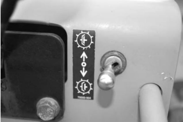
Figure 9.11 A pull-to-engage toggle switch reduces the likelihood of inadvertent activation.
