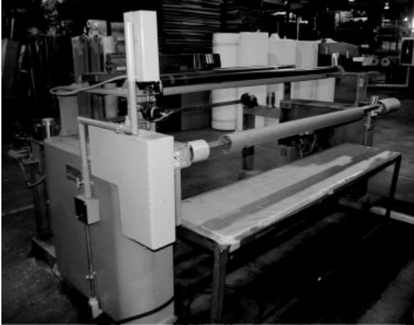
Figure 9.7 Light beams can be used to protect the operator from moving parts.
