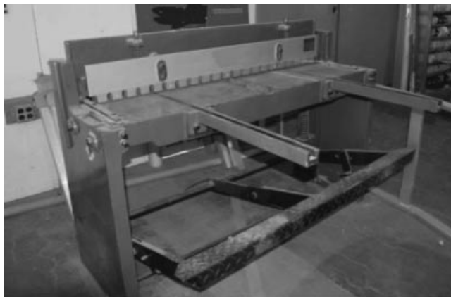
Figure 9.15 Finger guards provide operator protection for this manual foot shear.
