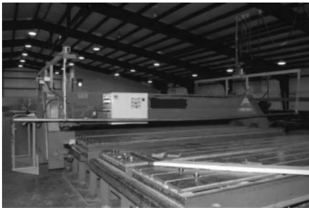
Figure 9.9 A safety bar on a truss machine. Unlike the safety bar shown in the photograph, a safety bar should be of rigid construction and have redundant limit switches.
