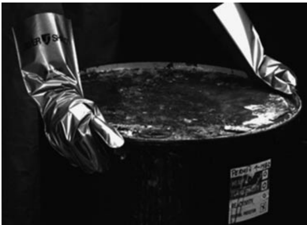
Figure 13.2 Laminate chemical-resistant gloves provide protection from a wide array of chemicals but little cut and abrasion resistance (OSHA, 1996).
