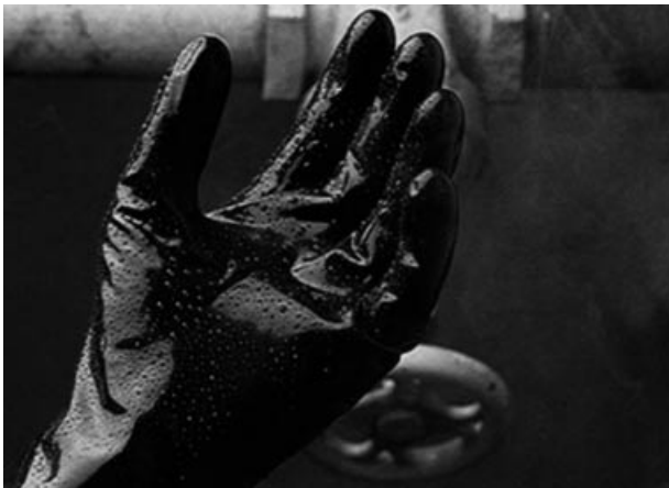
Figure 13.4 Chemical-resistant gloves made of Viton are highly resistant to chlorinated and aromatic solvents (OSHA, 1996).
