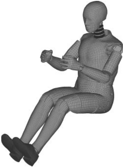
Figure 17.17 Hybrid III 50th percentile FE model. (Reproduced with permission of Humanetics Innovative Solutions, Inc.)
