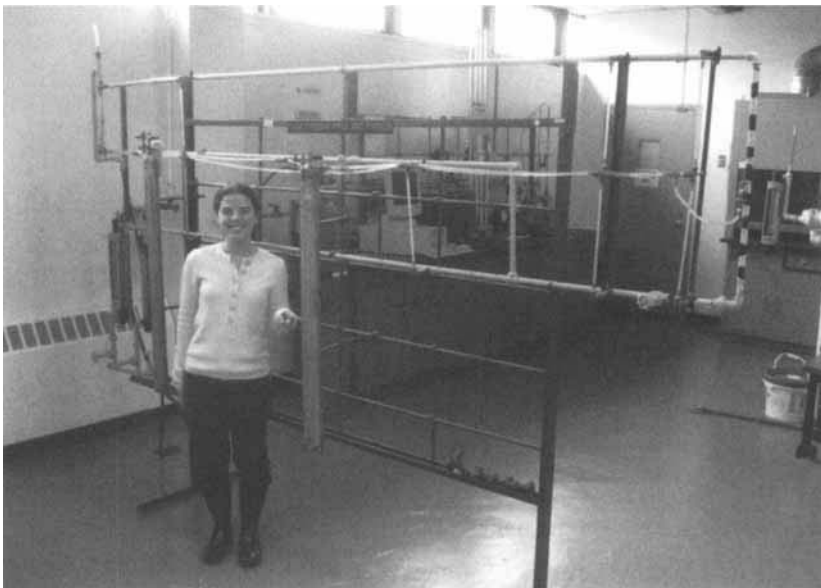
Figure 18.7 Flow through pipes and fittings.
