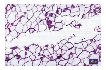
**Fig. 6.6** Fracture through cell walls of fresh vegetable. Reproduced with permission from Lillford (2000) The materials science of eating and food breakdown. *MRS Bulletin* 25(12), 38–43. Cambridge University Press.
