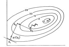
Figure 10 The Steepest Descent Method.
