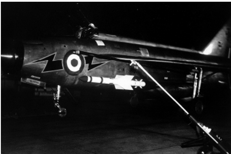
Figure C.5 A Lightning Mk 1A of No 111(F) Squadron undergoing night OTR (operational turn round.) Note the radome in the nose of the aircraft, the Firestreak Missile with protective covers, center, and the refueling probe at the top of the roundel (photograph by author).
