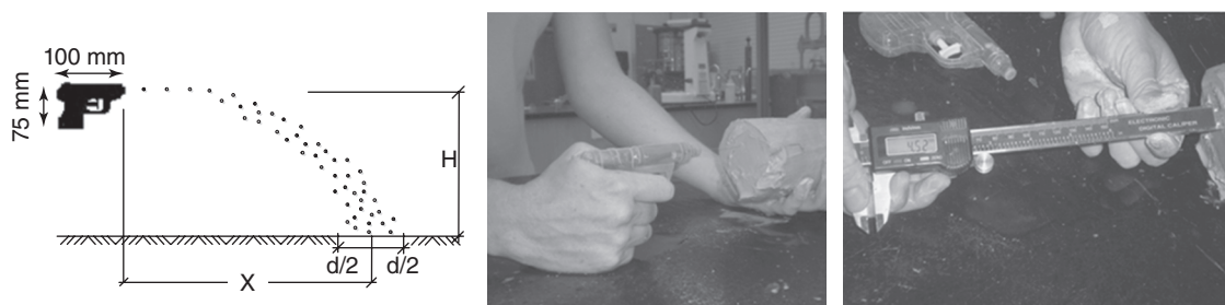
Figure 7.29 Pocket erodometer test.
