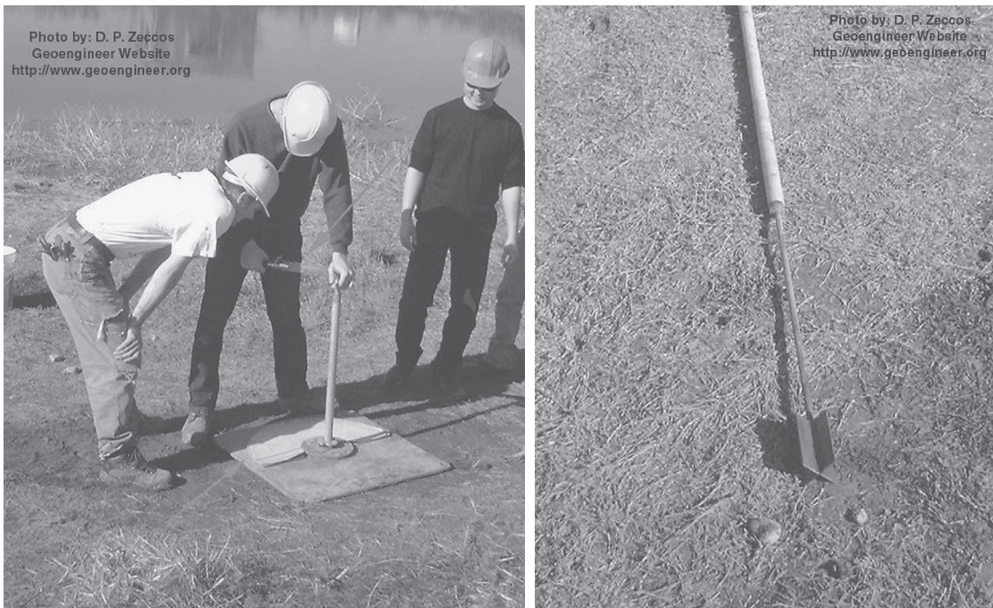
Figure 7.19 Field vane shear test. (Courtesy of Dr. Dimitrios P. Zekkos.)
