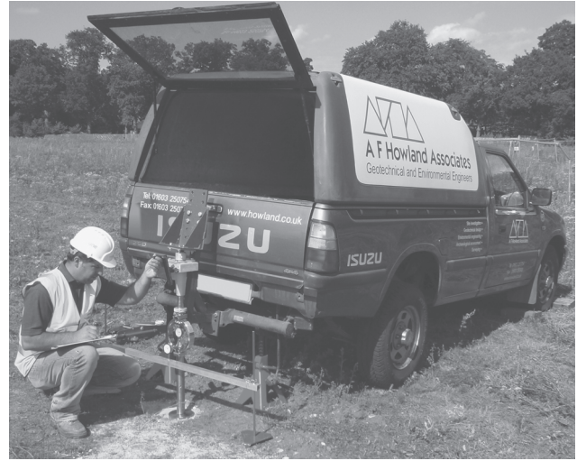
Figure 7.27 CBR test in the field. (Courtesy of A F Howland Company.)
