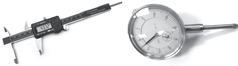
Figure 9.12 Mechanical devices to measure displacement: (a) Calipers. (b) Dial gage.
