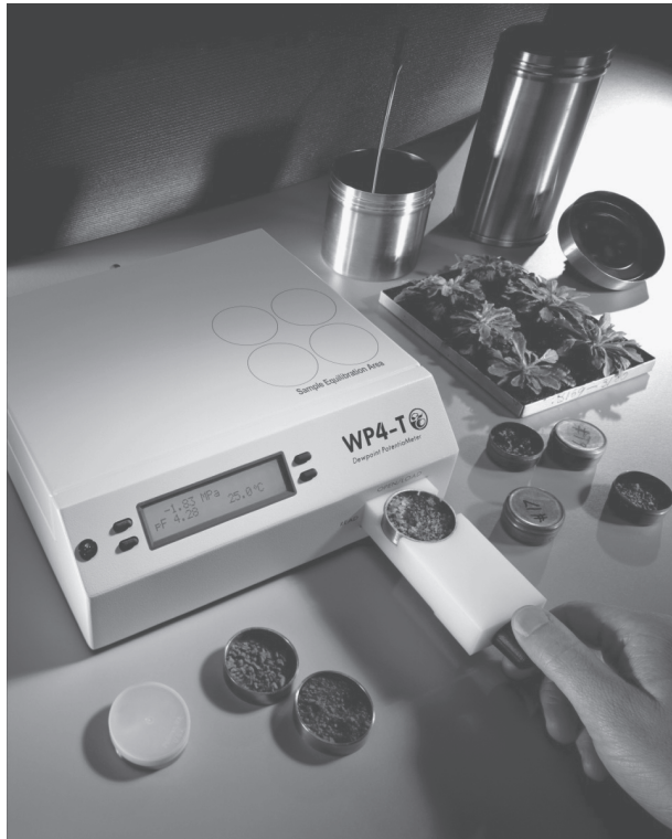
Figure 9.7 Chilled mirror psychrometer. (Photo courtesy of Decagon Devices, Inc.)
