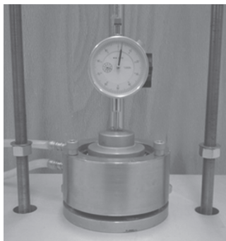
Figure 9.33 Swell test equipment.
