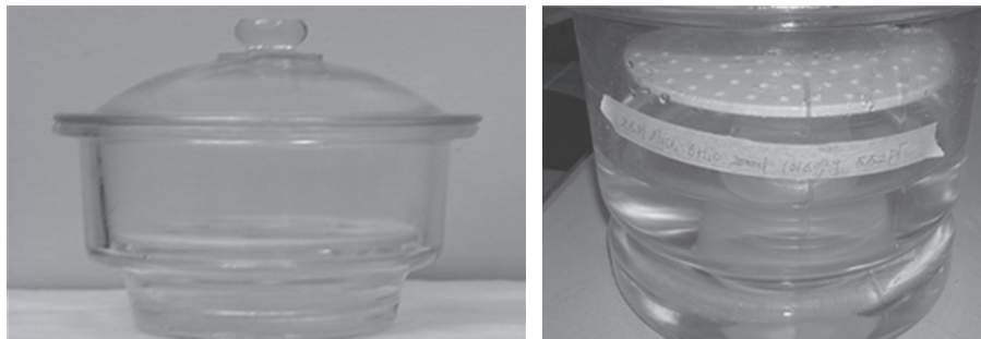
Figure 9.11 Salt solution equilibrium containers for water tension determination.
