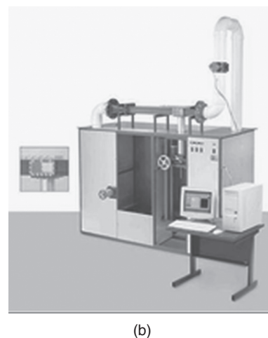
Figure 23.3 Erosion function apparatus to measure erodibility (Briaud et al. 1999).
